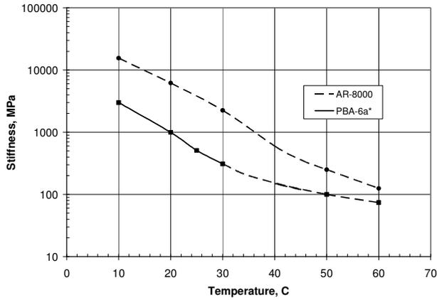
**FIGURE 4. Mix stiffness versus temperature; mixes containing AR-8000 and PBA-6a\* binders**
