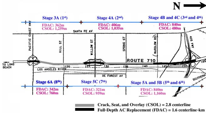
**FIGURE 7. Contractor's revised staging plan (sequence of 55-hour weekend closures shown in parentheses).**
