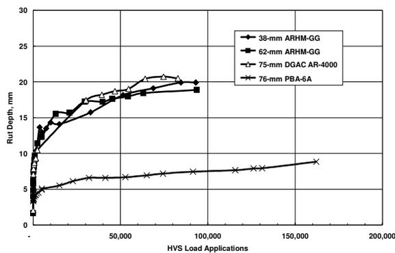
**Figure 6. Rut depth versus HVS load applications with 40 kN load on dual tires at 50°C (122°F).**
