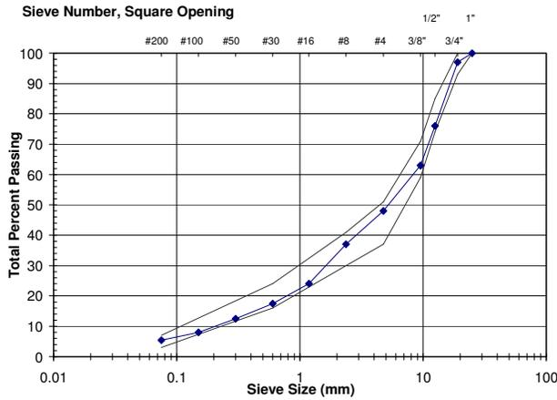
**FIGURE 2 Aggregate grading.**
