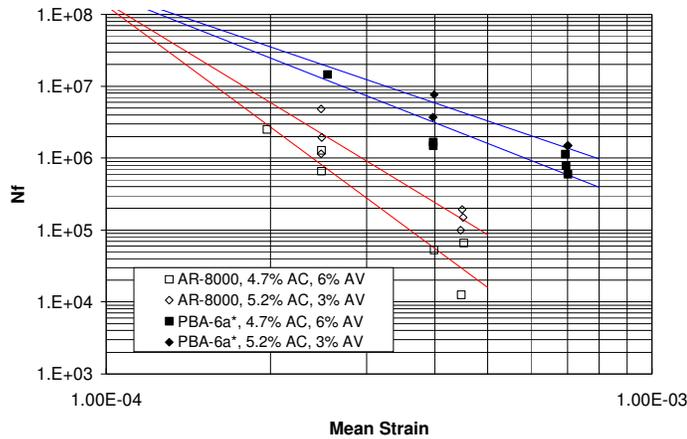
**FIGURE 3 Controlled-strain fatigue tests at 20°C (68°F), 10 Hertz frequency.**
