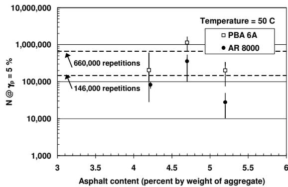
**FIGURE 5. Repetitions to 5 percent permanent shear strain,  $N_{\text{supply}}$ , versus binder content; tests at  $50^\circ\text{C}$  ( $122^\circ\text{F}$ ).**
