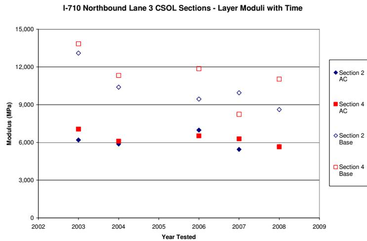
**b. Crack, seat and overlay sections**
