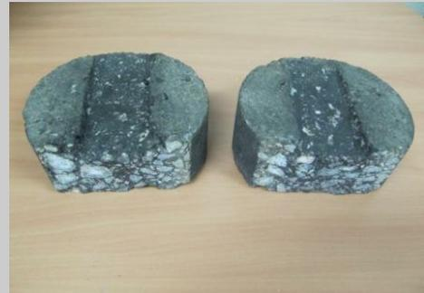
*Samples taken from a completed HWT test.*
