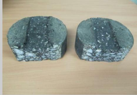
*Hamburg Wheel Track post-test samples.*
