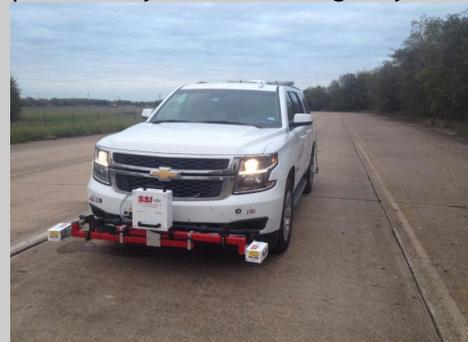
***A vehicle with inertial profiler equipment mounted on the front to measure pavement smoothness.***
